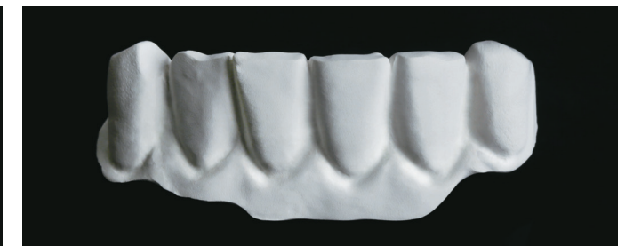
The result of 90° milling
